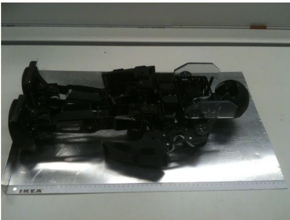
(a) Laying robot upright on measurement device.
