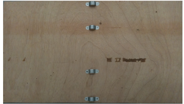
(b) Aligning pipe straps on the wooden board
