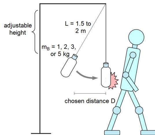
Figure 5: Setup for the push recovery challenge.
